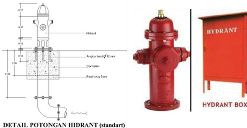
Gambar 3.124 Tipikal Hydrant Halaman (Pilar)
